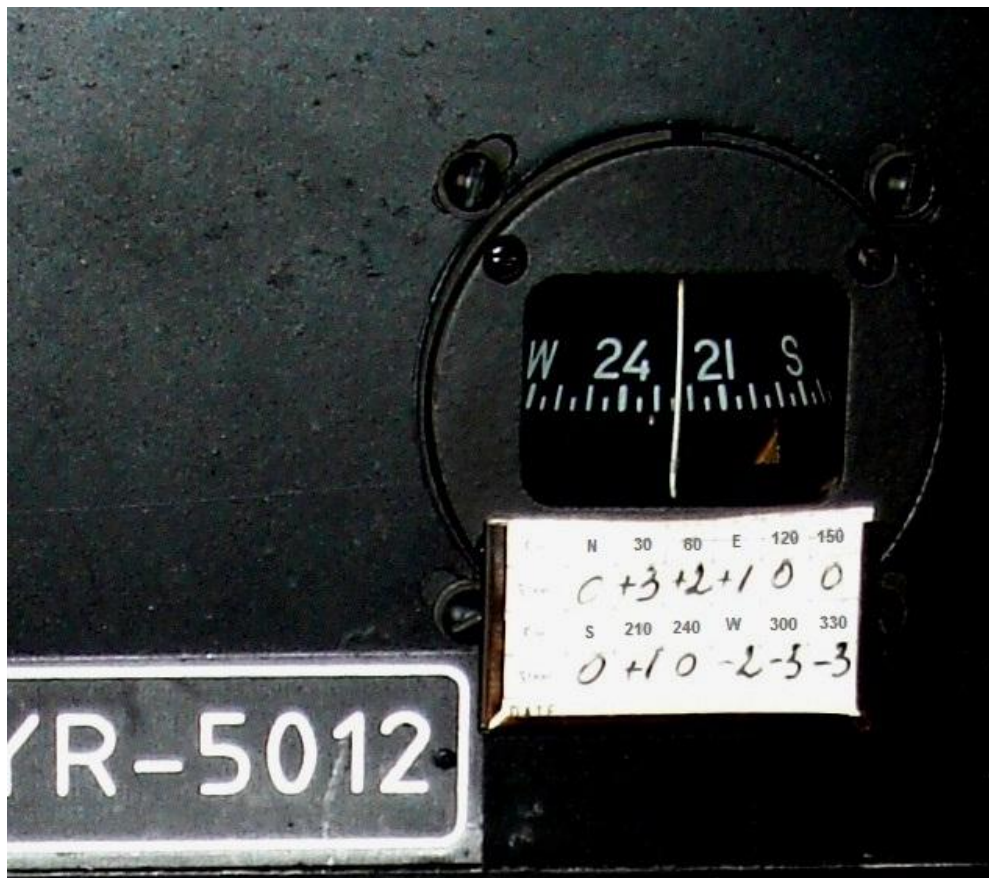
Fig. 4.25. Busola Aerostar Festival si cardul de compensare a busolei
